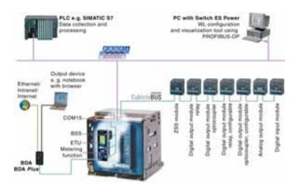
The modular design of the system allows the retrofitting of communication functions at any time. This also allows trouble-free and local upgrading of a WL Circuit Breaker that does not yet have commun-
